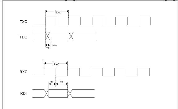
The MAS9140 has inverted RXC and TXC clock inputs. The data is shifted out to TDO with falling edge of XTXC and data is read in from RDI with rising edge of XRXC.
